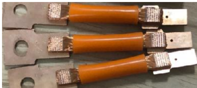
10cm长70mm 2 铜线两头焊接
